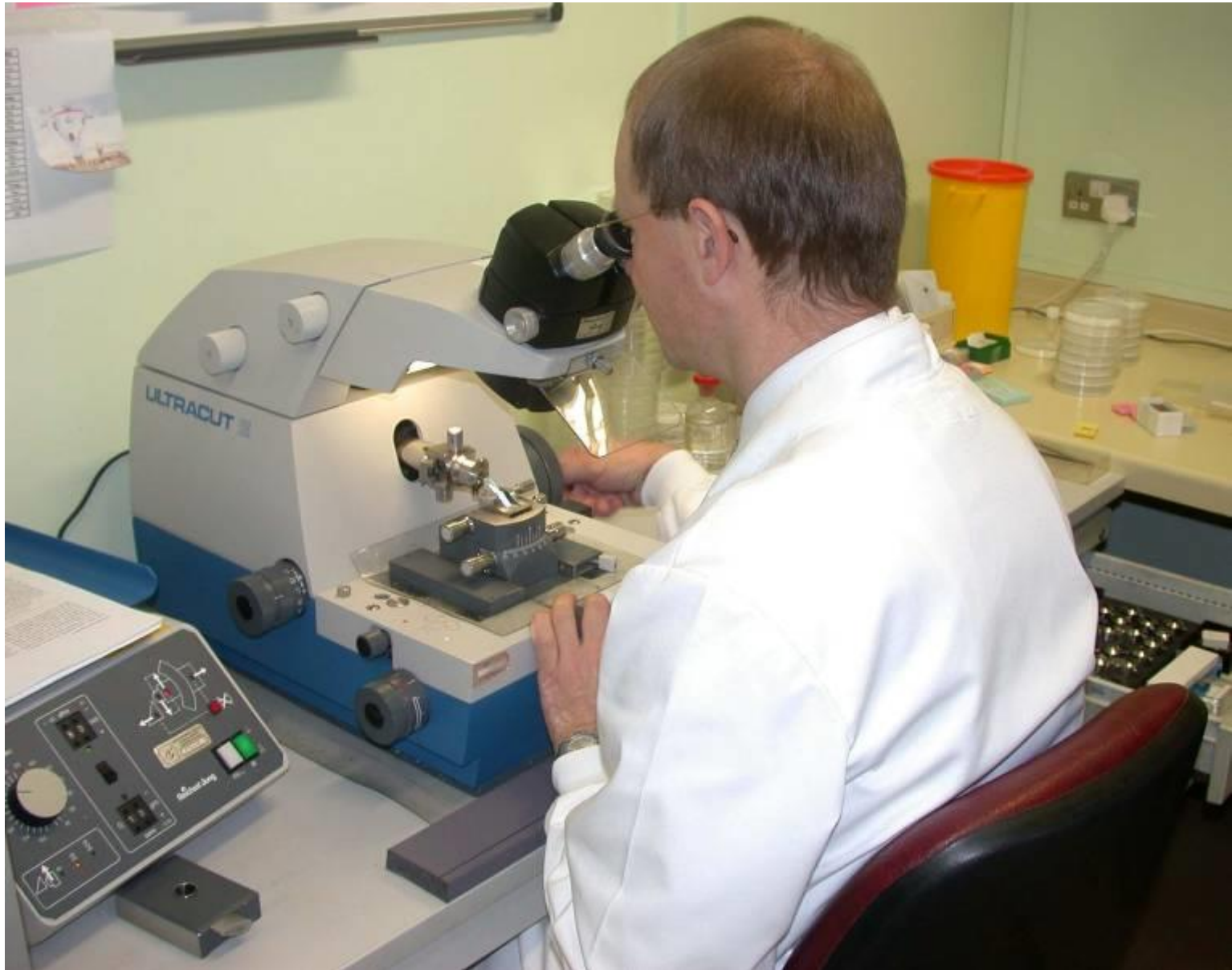
Ultramicrotome in use by BE Wagner
