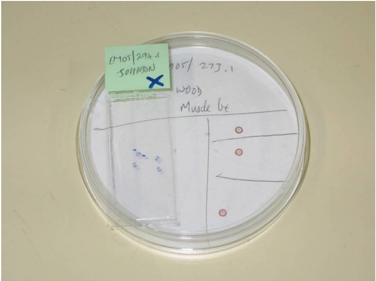
Toluidine blue stained section on glass slide and thin section on copper grid
