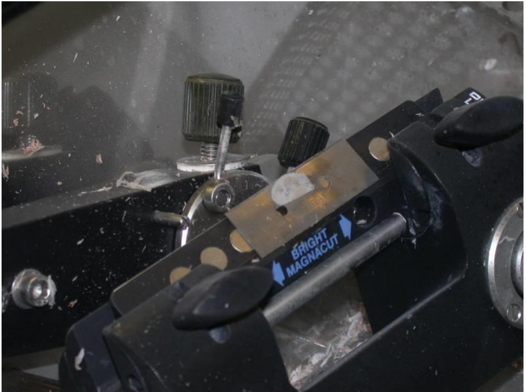
Frozen section sitting on knife before being picked up on glass slide
