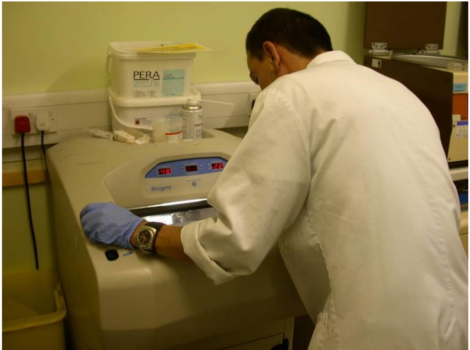
Cryostat (microtome within freezer) for production of frozen sections
