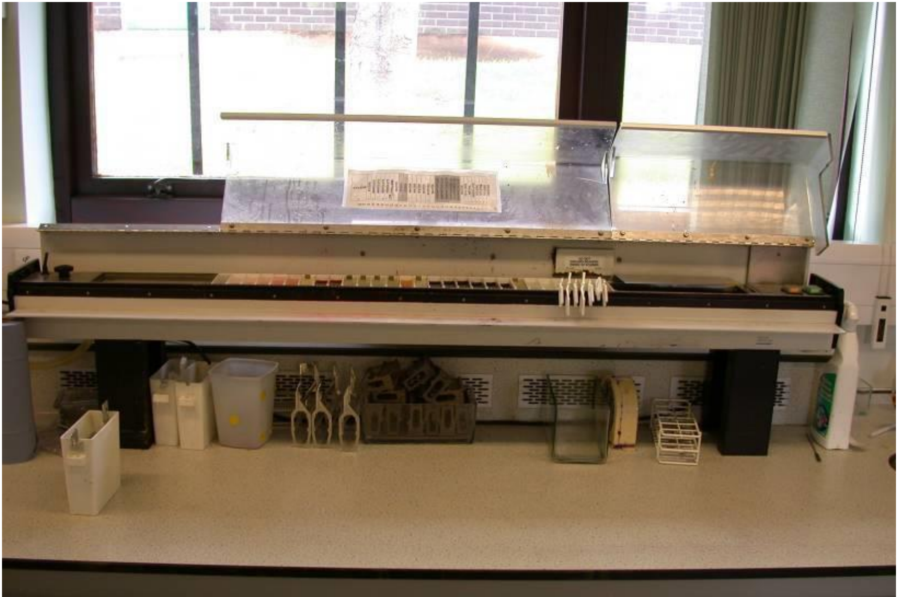
Automated Haematoxylin and Eosin (H&E) staining machine
