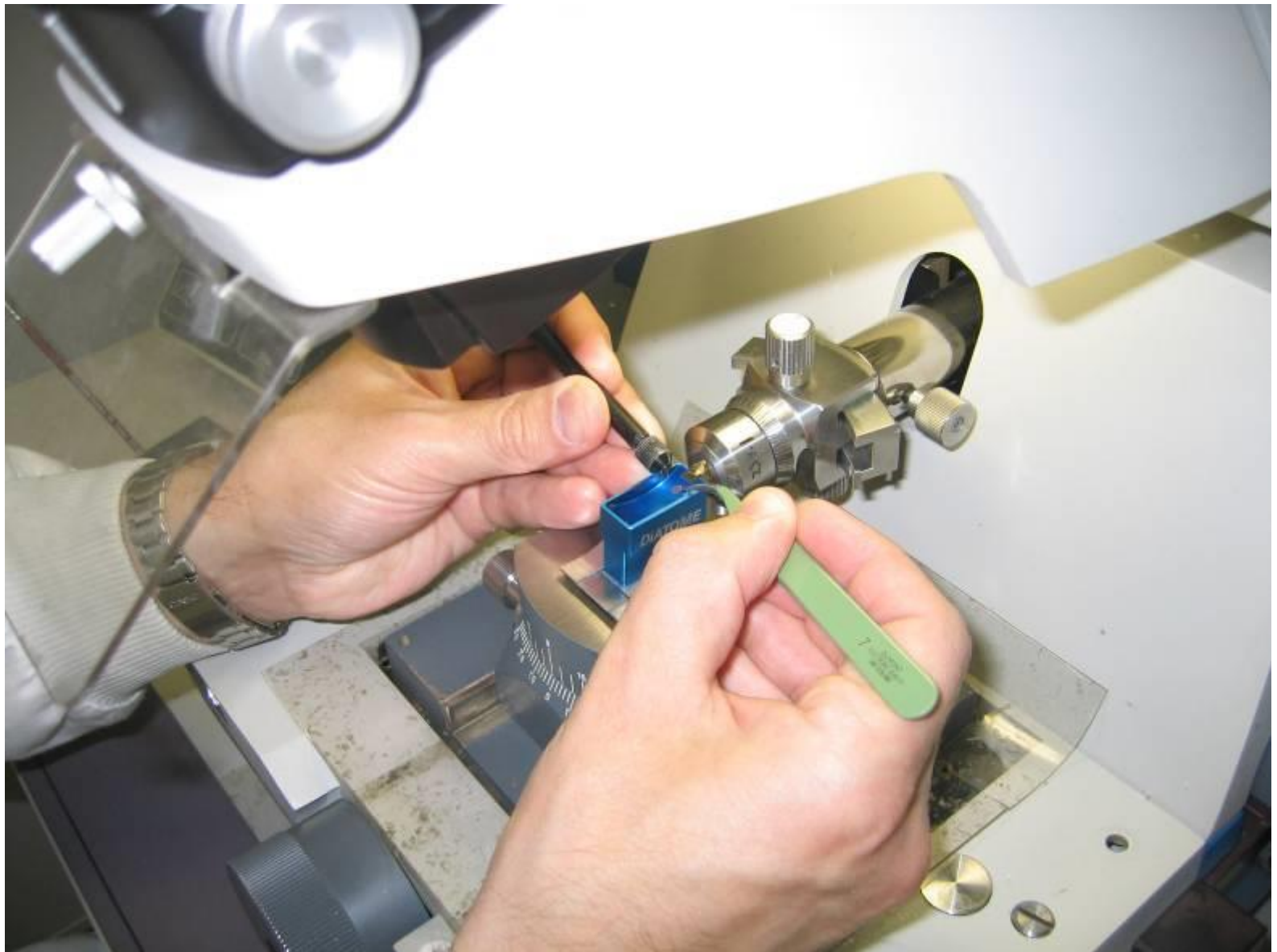
Thin sections picked up on copper grids (held using jewellers forceps) , sections manipulated with eyebrow hair fixed at end of black metal rod. All manipulation done whilst looking down stereo microscope.
