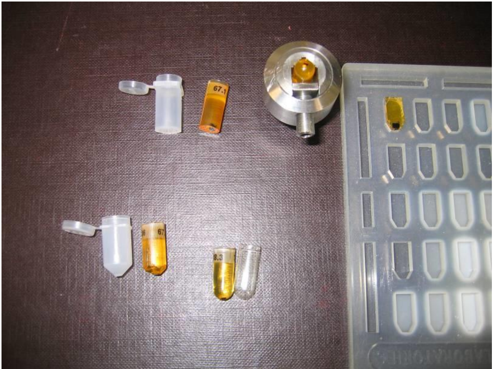
Different moulds for resin blocks
