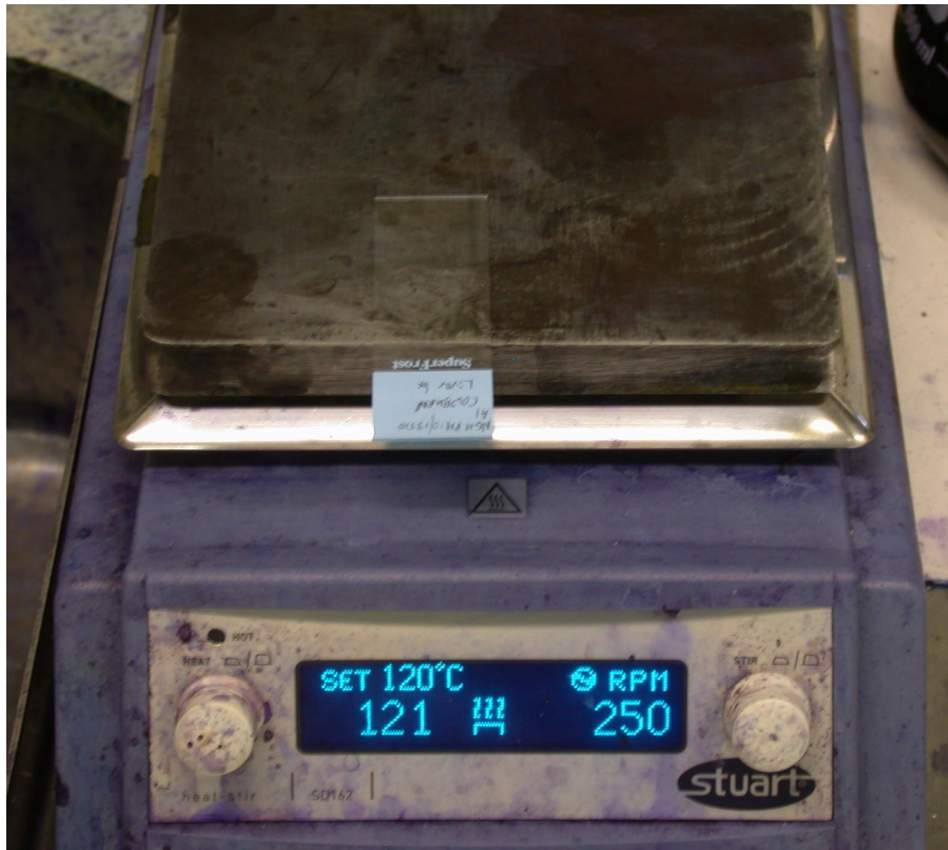
Section flattened using heat
