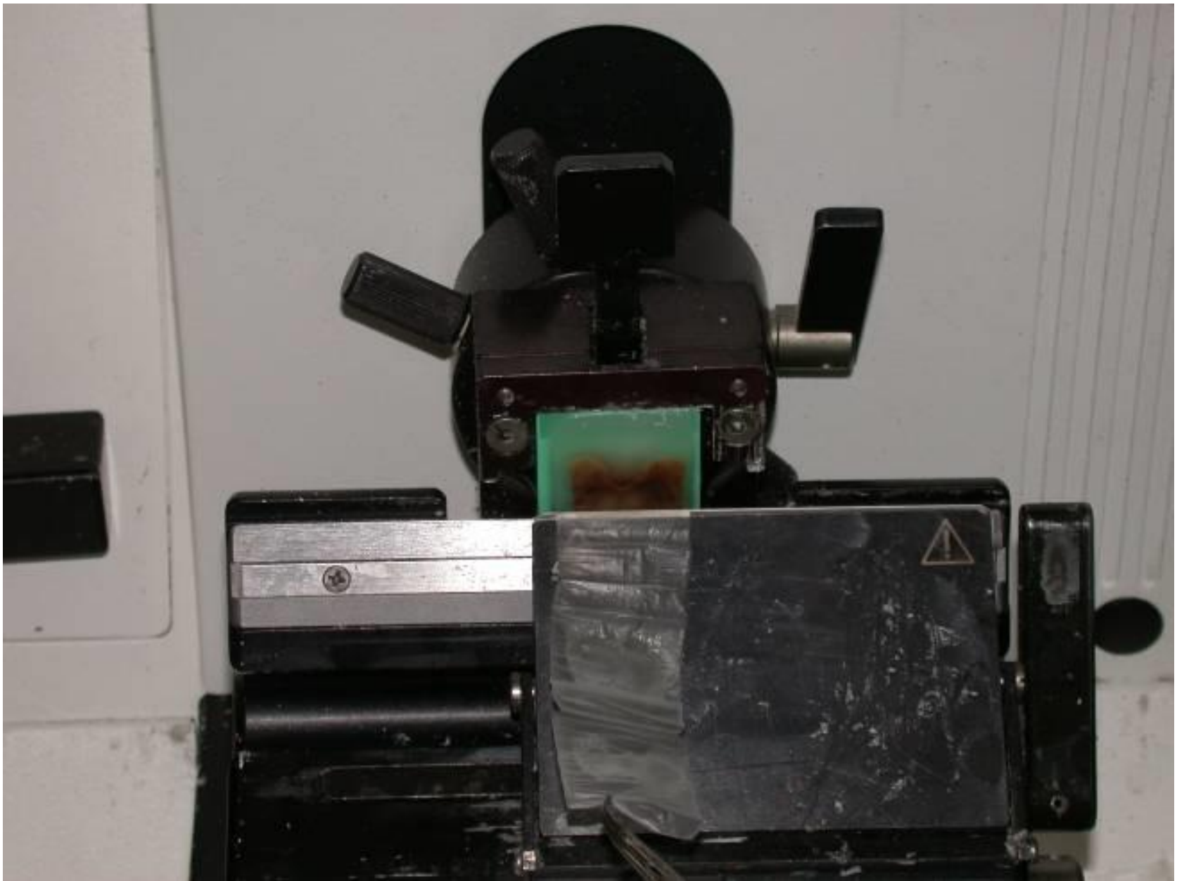
Paraffin sections being cut on rotary microtome – using disposable blade
